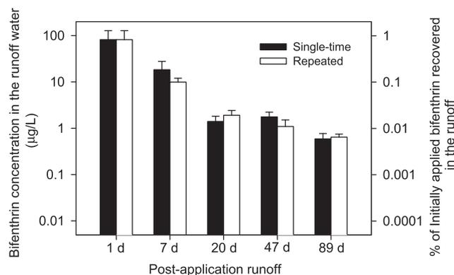
**Fig. 1** – Levels of bifenthrin in the runoff following simulated single-time or repeated precipitations at  $26.2 \pm 2.7$  mm/h ( $n = 4$ ). The results are expressed as bifenthrin concentration ( $\mu\text{g/L}$ ) in the runoff water and percentage of the initial application rate.
